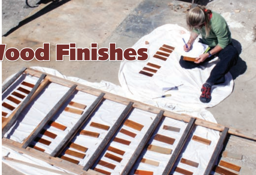
PS’s search for the ideal wood finish continues with a six-month checkup, rating panels for coating integrity, gloss retention, and color retention.
