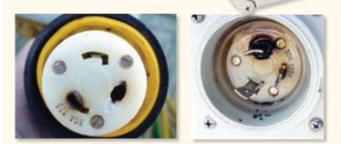
Once discoloration is visible at the plug face (left) or shoreside socket (right), you'll typically find more damage inside. If left uncorrected, this could create further damage to the system and even lead to a fire.
