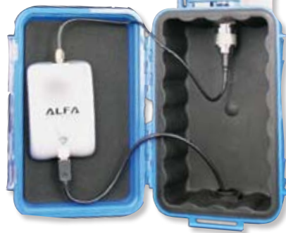
The Wirie's insulated and watertight box protects the Alfa Wi-Fi adapter.
