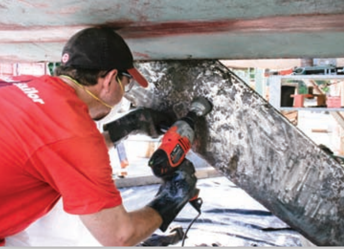
The keel on PS's 35-year-old O'Day Javelin is prepped for a coatings test (above). Reader Dick Paden's keel weeps (right).
