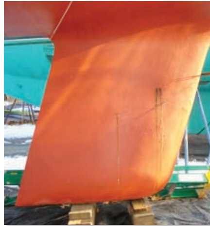
The keel on PS's 35-year-old O'Day Javelin is prepped for a coatings test (above). Reader Dick Paden's keel weeps (right).
