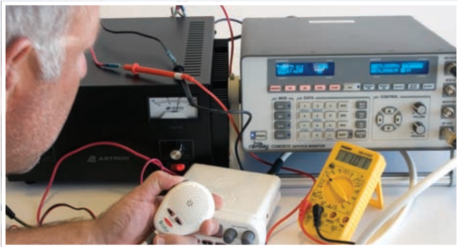
Bench testing evaluated each radio's transmitter power, frequency accuracy and stability, and receiver sensitivity.
