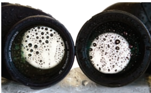
Testers sprayed water on the lenses to test the Commander XP's hydrophobic coating (left) against the coatings of the other binoculars, like the Fujinon (right).
