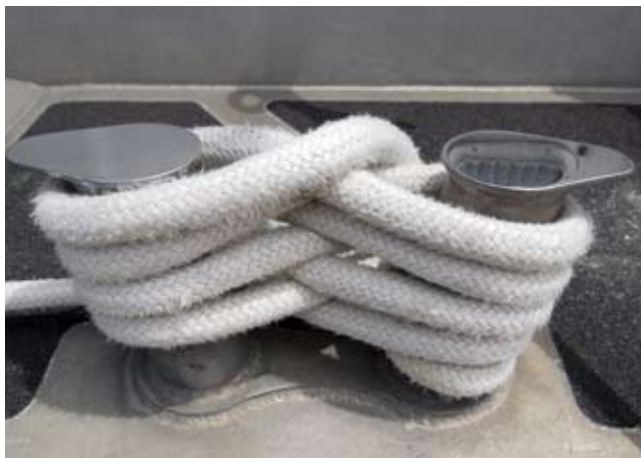
This heavy-duty bitt on the Coast Guard Rescue 47 cutter is also found on many oceangoing yachts. The bitts can accommodate multiple turns and thick-diameter lines.
