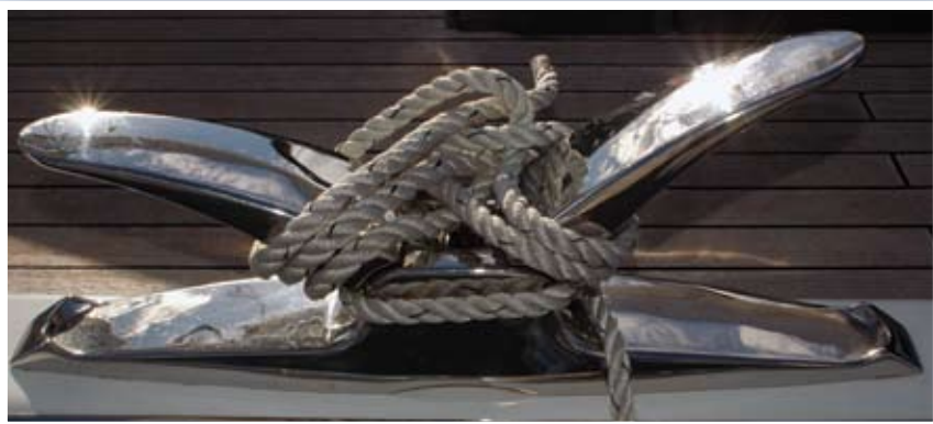
The investment-cast fold-up cleats found on new Oyster yachts (holding a fender here) present a good combination of beauty and functionality.
