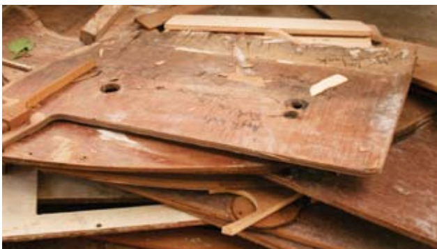
..... This pile of water-damaged teak was key to the refit. Formerly Satori's cabin innards, the wood was used as patterns for cutting the new settees, nav table, V-berth, shelves, galley sink shelf, etc.
