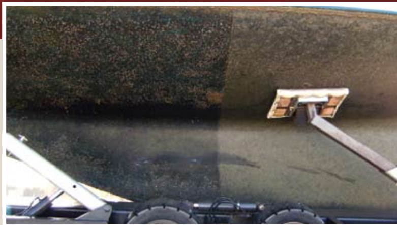
After 20 months in the water, both Flexdel Aquaguard (left) and Pettit Hydrocoat (right) showed significant growth at haulout. Hydrocoat had more slime but fewer barnacles.
