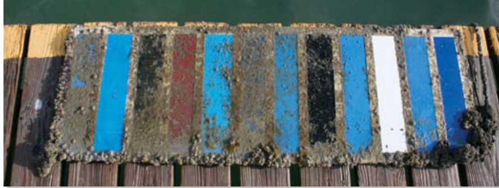
Most of the slime on the test panels washed away with a bucket rinse, and all but a few paints proved very effective at combatting hard growth for six months.
