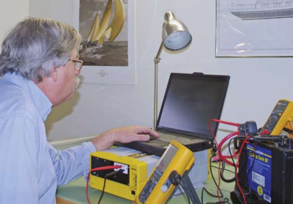
Testers used a Fluke meter connected to a laptop to evaluate waveform and to assess the level of harmonic distortion that the true-sine wave inverters produced.
