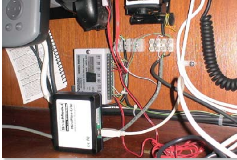
To evaluate the ShipModul MiniPlex Lite, we interfaced our Dell Latitude D620 laptop (Windows XP) with a C-Series Raymarine chartplotter and an old Garmin GPS 48. A low-speed Noland NC42U multiplexer, is in the background.
