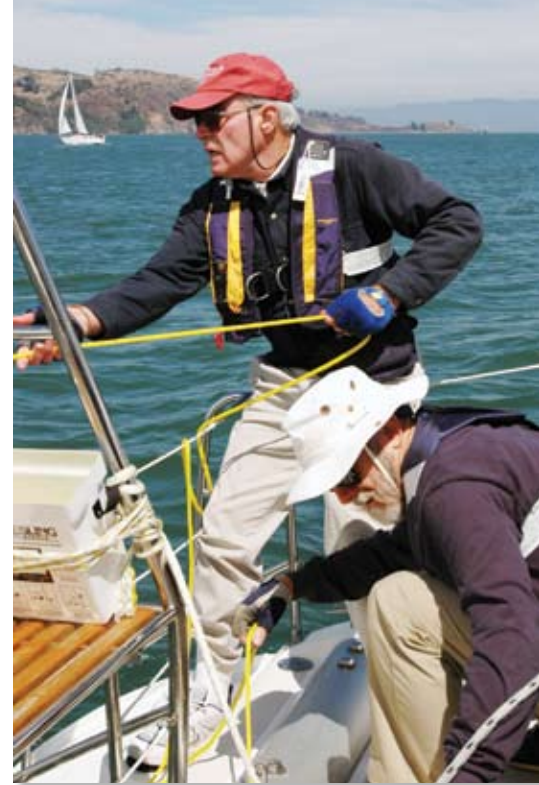
Once the victim is securely connected to the Lifesling, crew can haul him to the boat, hand over hand or using winches.
