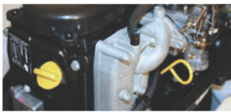
Mercury and Tohatsu oil fill and dipstick
