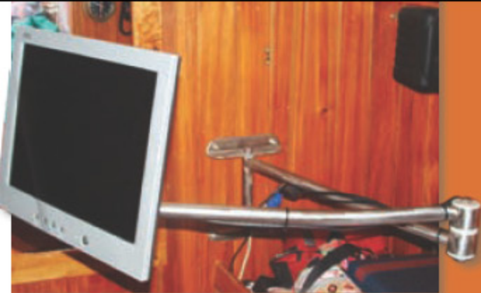
The AOC monitor (left) pivots on a home-made arm. The enclosure (right) is larger than necessary (compare to cassette player).
