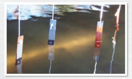
The saltwater test strips were suspended from a dock, where they faced the daily tide cycles.
