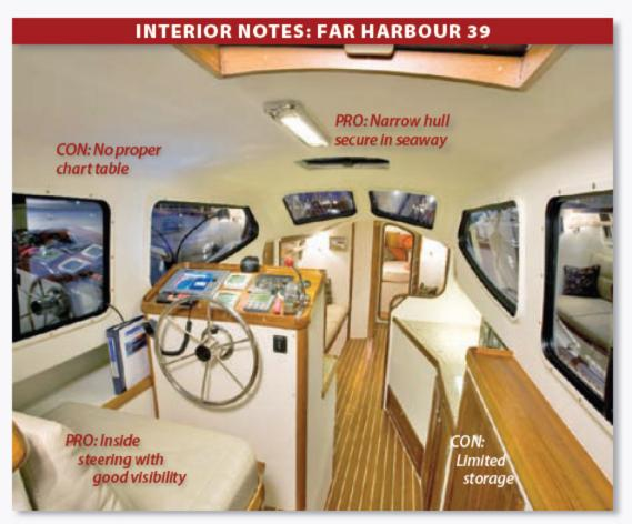
A wide-angle lens makes the Far Harbour 39 appear wider than it actually is. While the narrow living space imposes restrictions at anchor, the tight layout becomes an asset in a seaway. No matter where you are in the hull, there's a place to brace yourself. Not shown is the drop-leaf table in the production models.
