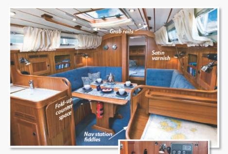
The interior of the Hallberg-Rassy 342 shows a good approach to offshore passagemaking with not too many compromises. Details like twist open drawer latches, ample grab rails and fiddles, and two sea berths coincide with a passagemaking purpose. The most apparent trade-off is a tight nav station (right), a necessary evil for having an aft head. The aft cabin (not pictured) is tight, but livable.
