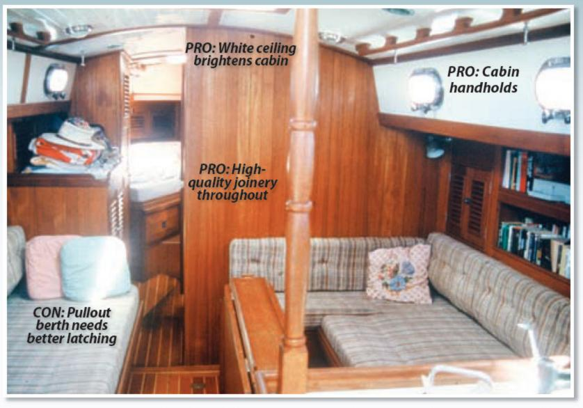
Both the Shannon 37 (above) and the Shannon 38 followed two basic interior configurations that could be customized. One layout featured an aft head; the other placed the head forward. Because of the centerboard, water tankage on the Shannon 37 is located beneath the settees port and starboard. On the 38, tankage is beneath the cabin sole in the keel, allowing more room for stowage beneath the settees.
