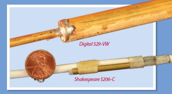
Testers found that the radiating element of the \$36 Shakespeare 5206-C is siginificantly thinner than that of the \$149 Digital 529-VW.
