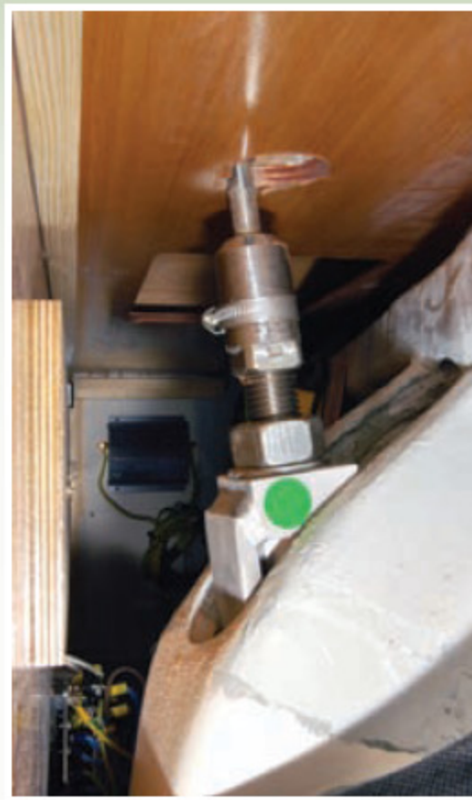
Tie-rods connect chainplates to massive FRP gussets, transferring rig loads to the hull.
