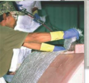
A laminator applies a layer of chopped strand mat to the underside of a cored cockpit well (inverted here). The core is bedded in a resinrich mixture of chopped strand mat. Hand-lamination requires more resin to eliminate voids. Although reaching panel consistency is nearly impossible, careful application can result in a strong, durable hull.
