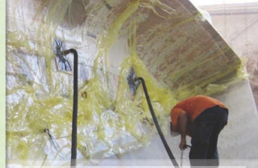
A Tartan hull takes shape at the factory in Fairport, Ohio. Epoxy-impregnated, unidirectional E-glass fabric followed by ATC Core Cell foam and additional laminates of E-glass are vacuum-bagged at 1 atmosphere. The hull is then cured in a temperature-controlled oven.
