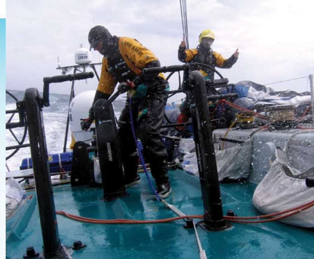
ABN One skipper Mike Sanderson, right, inspects his office. A short tether enables him to hook to a soft padeye in the hub of the wheel, preventing him from losing his grip on the wheel when water rushes aft.
