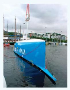
right the boat from a full inversion. Experience proved that it was only necessary to move the keel about eight degrees off the centerline before the boat would flip upright in an instant. To minimize the risk of injury to the crew, the crane was left loosely connected to the bulb during the test to slow down the righting of the boat.
