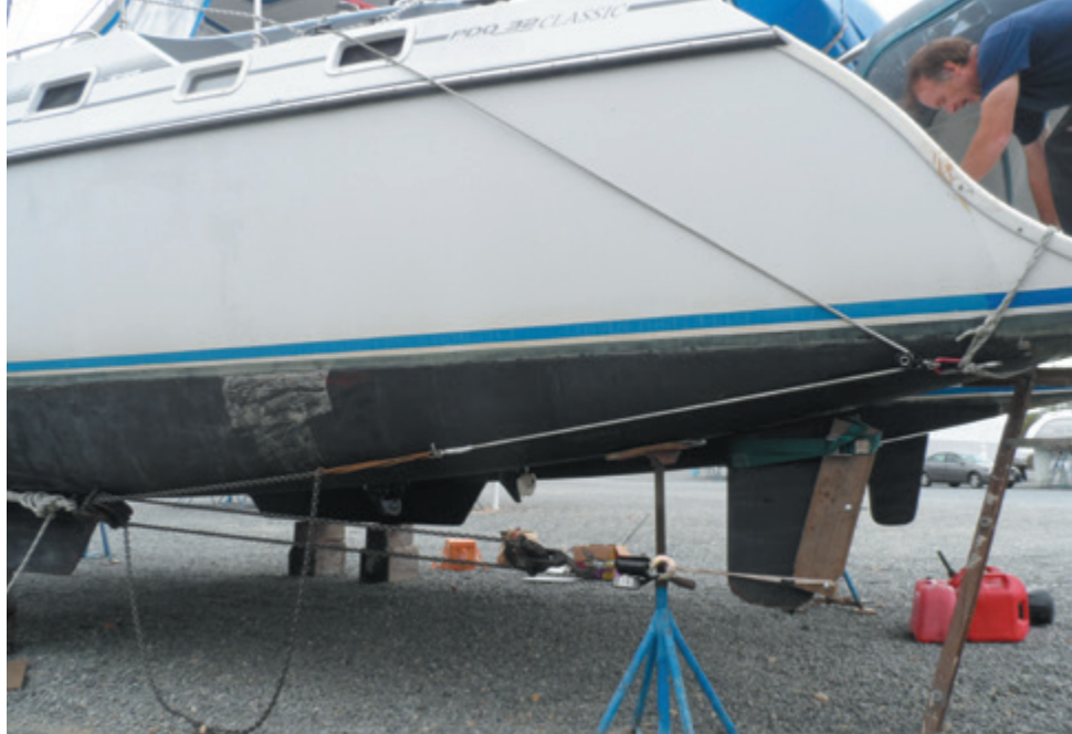
With a careful application of force and robust bracing, it is possible to straighten a rudder. Note that no forces were applied from points off of the boat.
