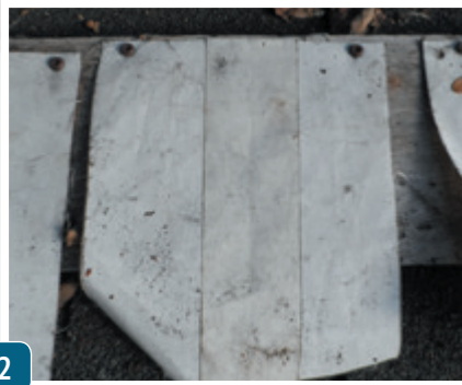
From left: 1. G-Flex hangs tough on polyester sail cloth and on Sunbrella. 2. Polyester tape, applied to both sides remains stronger than the sailcloth. The bond becomes better with time. 3. Polyurethane failed after one year, due to UV exposure.
