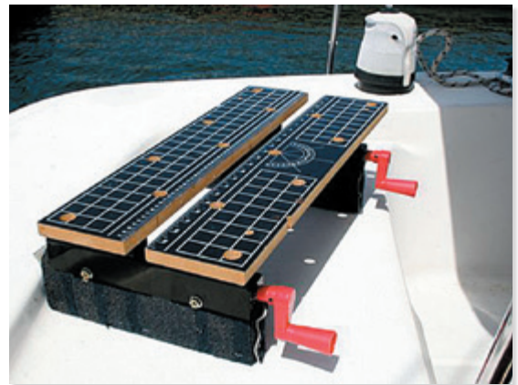
The Grizzly workbench, modified with some outdoor carpet on the bottom can be used for a variety of onboard projects. The Black and Decker workmate series benches (below), collapses and can provide a handy platform for boatyard work. Just don't leave it out in the rain.
