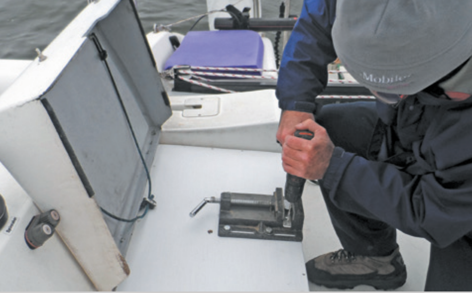
A horizontal-mount cockpit vise can be fitted into a piece of plywood that tucks neatly away when the boat is at sea, (see "A Handy Cockpit Vise is Ready in a Pinch," PS October 2019).
