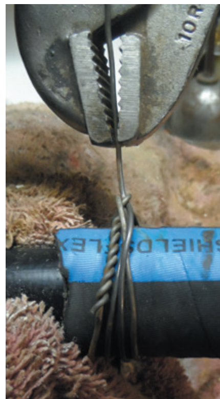
A few tight wraps is all it to replace a hose clamp or splice a wire
