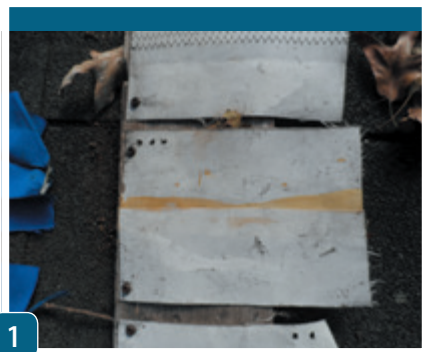
From left: 1. G-Flex hangs tough on polyester sail cloth and on Sunbrella. 2. Polyester tape, applied to both sides remains stronger than the sailcloth. The bond becomes better with time. 3. Polyurethane failed after one year, due to UV exposure.
