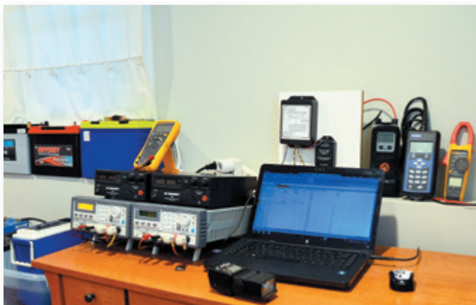
The Firefly carbon foam battery is among many that were tested and re-tested during our look at the effects of sulfation on batteries in the December 2017 issue.
