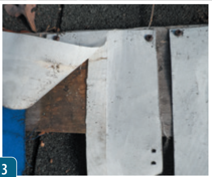
From left: 1. G-Flex hangs tough on polyester sail cloth and on Sunbrella. 2. Polyester tape, applied to both sides remains stronger than the sailcloth. The bond becomes better with time. 3. Polyurethane failed after one year, due to UV exposure.
