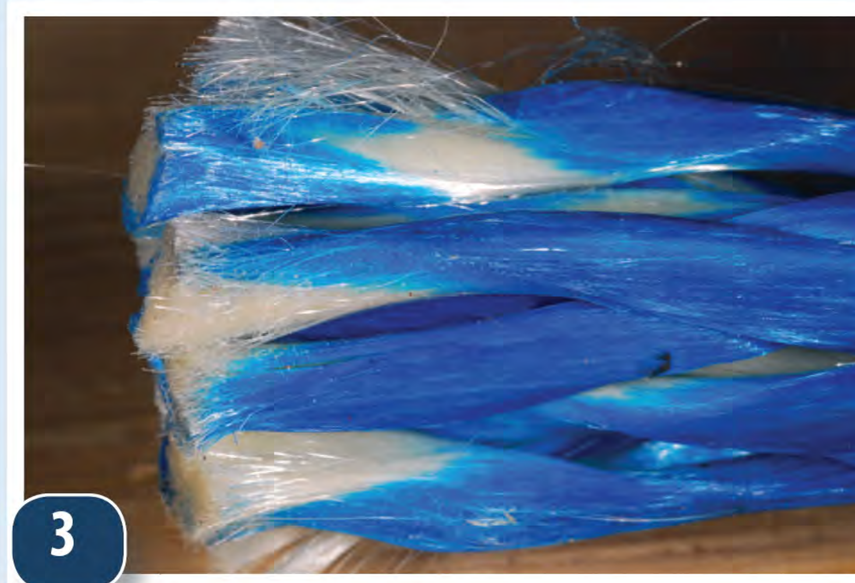
1. Yale Vizzion, with its Vectran core, resisted creep well. 2. A highly magnified tuft was the only sign of abrasion in the Amsteel. 3. The braided core of New England Ropes Endura is a blend of polyester and Dyneema. 4. The Novabraid XLE earned high marks as a sheet.
