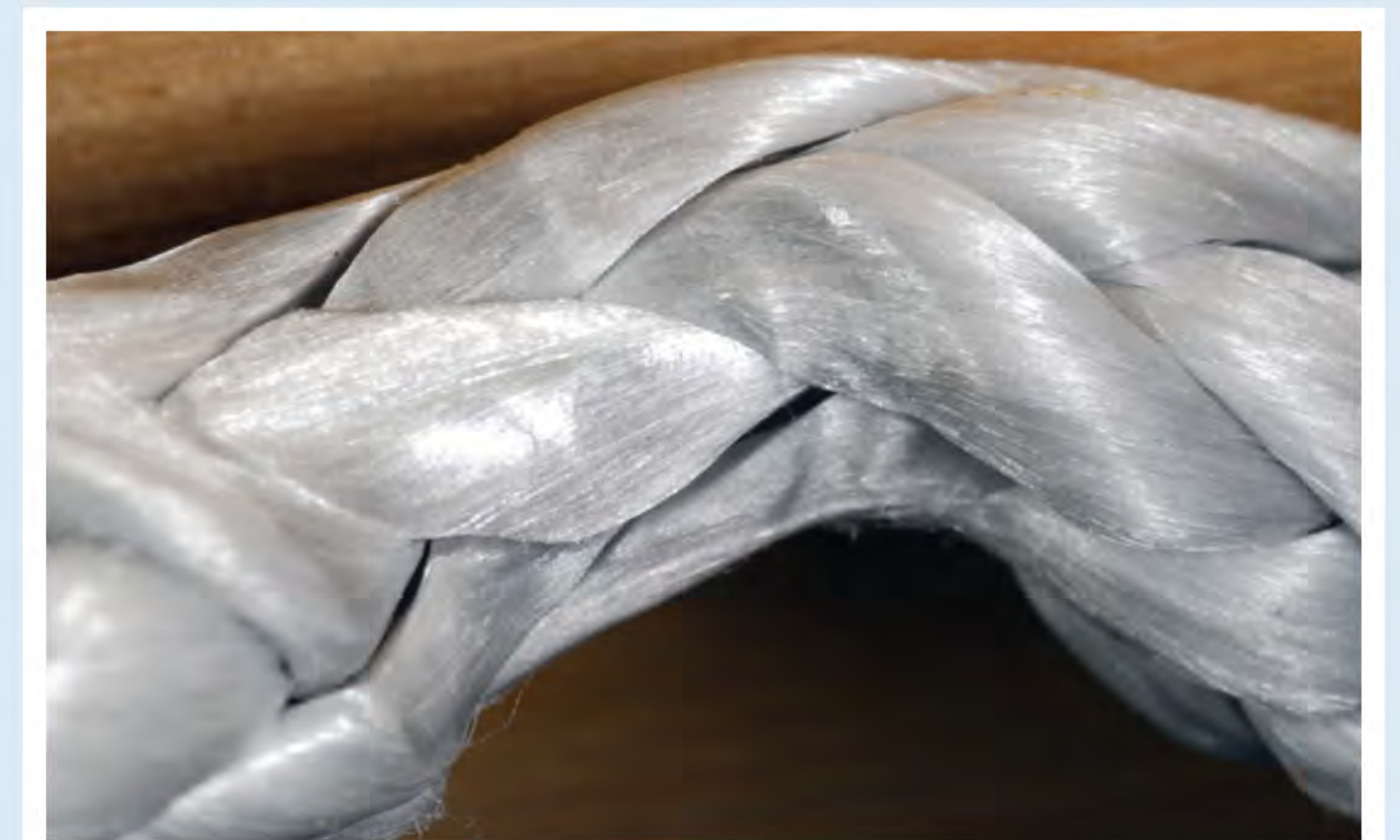
The bowline in the 3/8-inch diameter Amsteel didn't slip, but after tensioning, a permanent crimp remained where the knot was untied.
