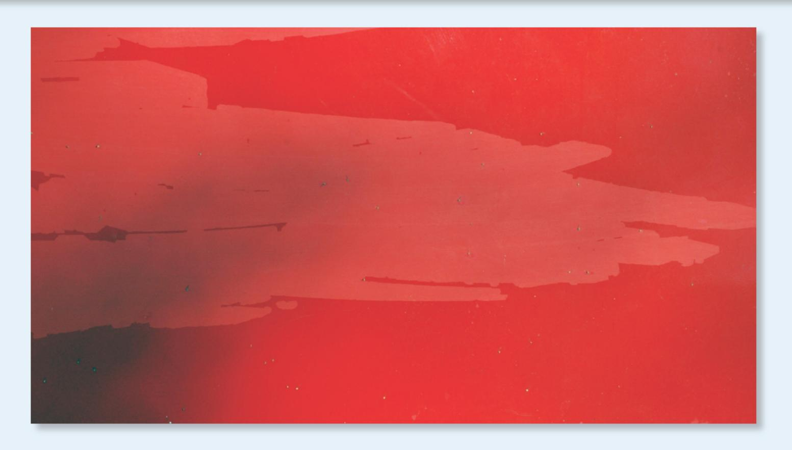
Despite basic pre-painting prep and de-waxing, the LPU lost adhesion shortly after application.
