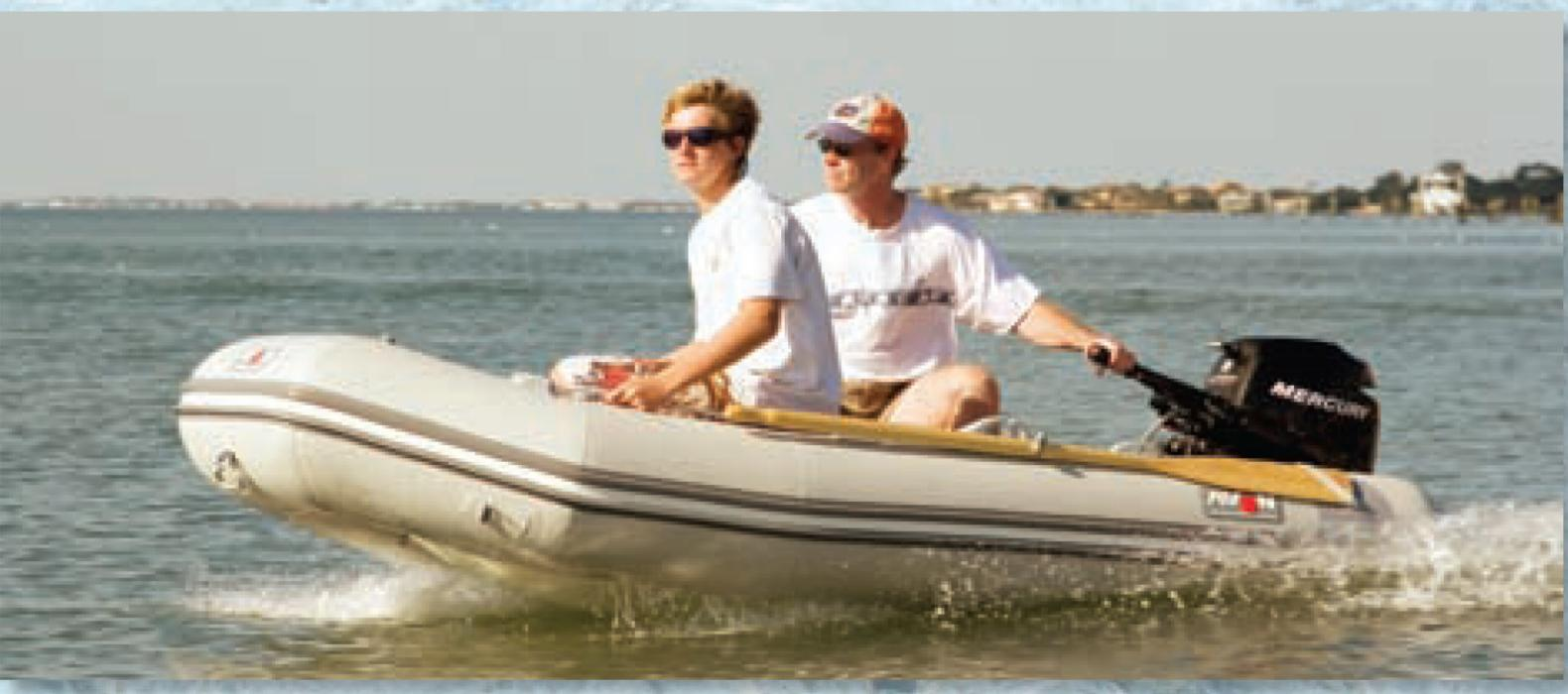
The Zodiac Zoom (top) has tubes made of a proprietary PVC material, Strongan, while the tubes of the Avon Rover Lite 310 (bottom) are Hypalon.
