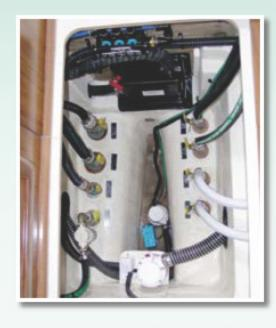
To minimize through-hulls, all raw-water intakes are led through a sea chest in the sump.
