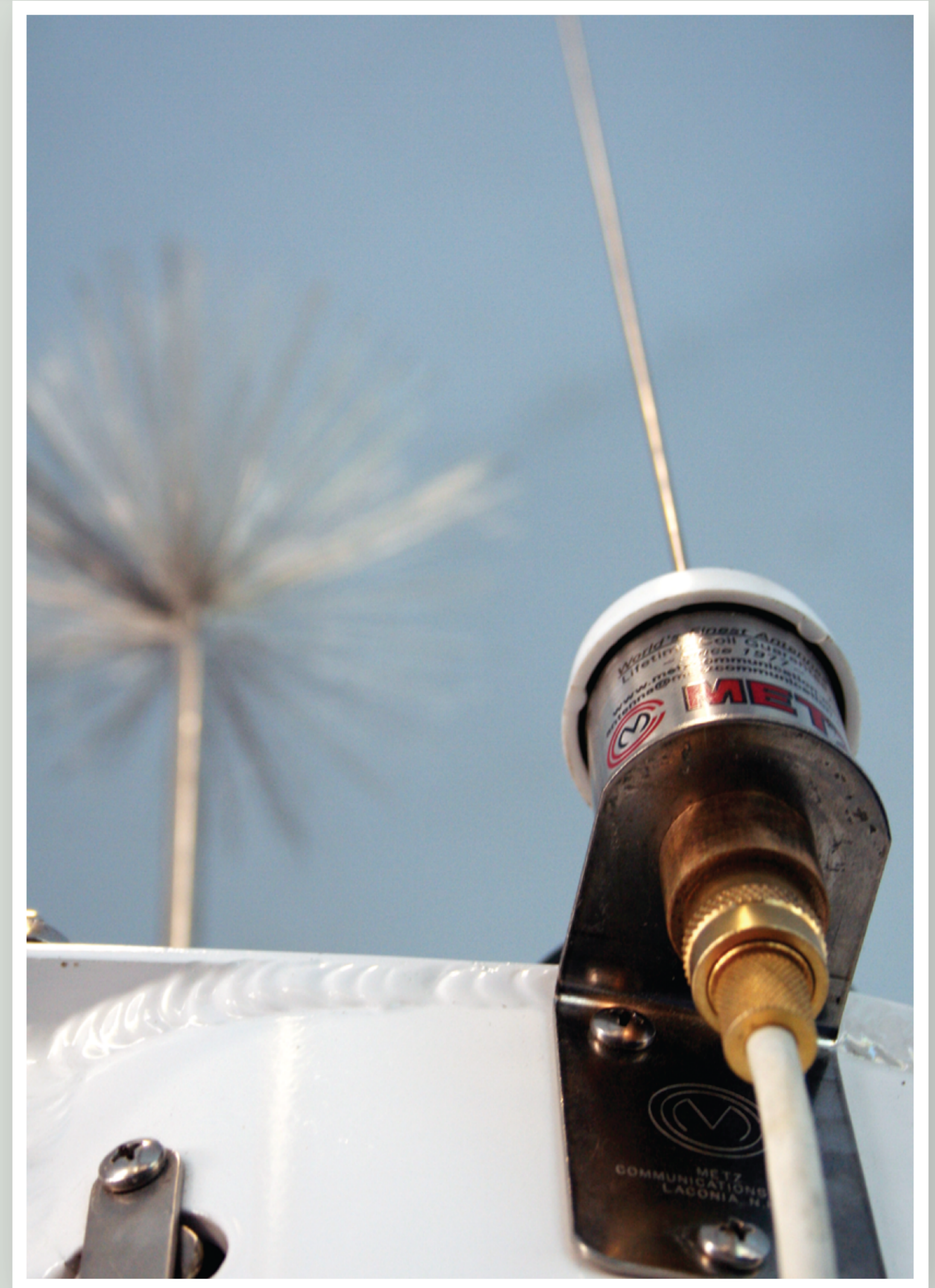
Mounting the VHF antenna on the mast and the AIS antenna on the stern rail will reduce possible interference.
