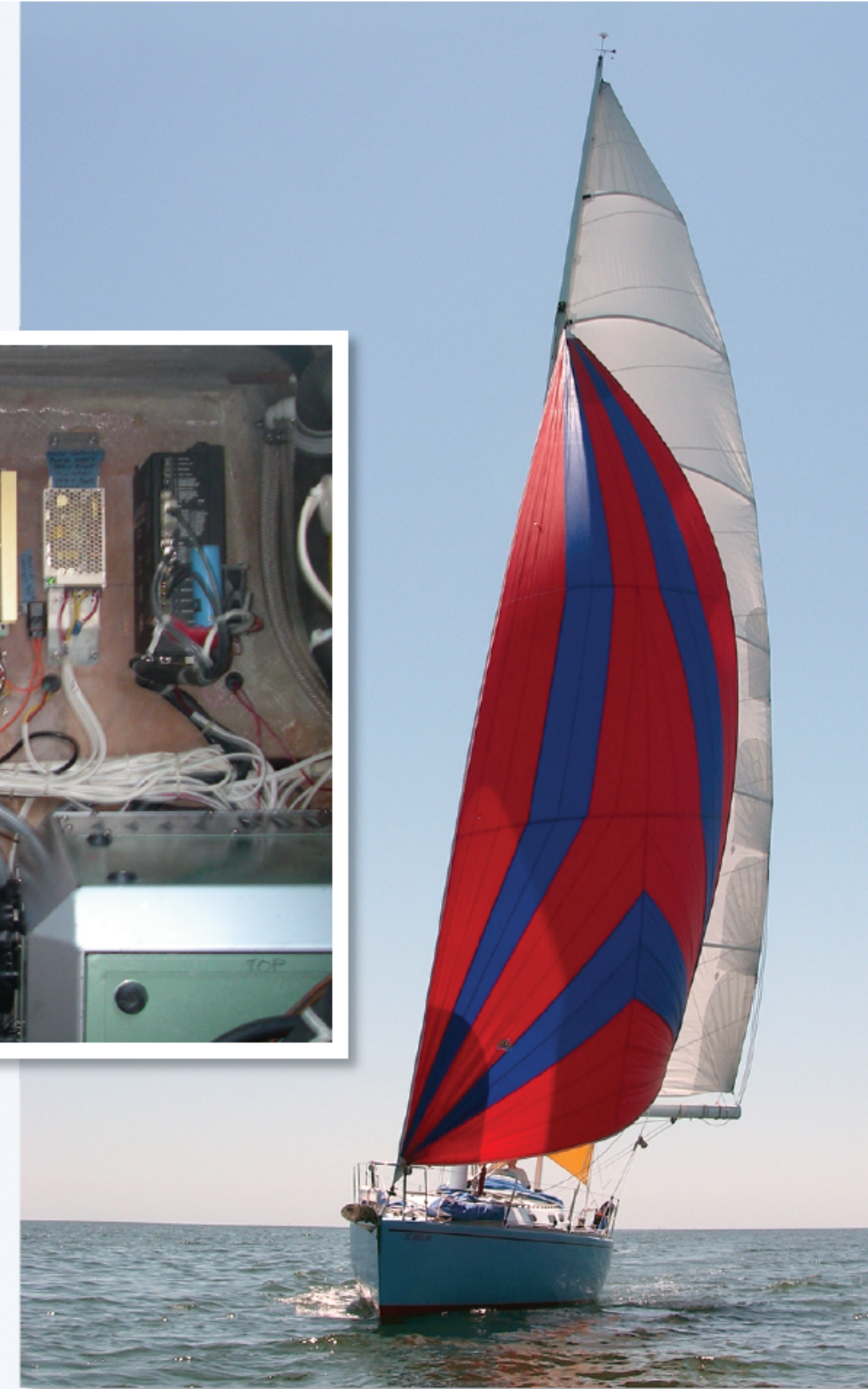
Joseph Huberman's custom Tom Wylie-designed Prestissimo (right) features Glacier Bay's 144-volt DC genset and related controls (above). The genset drives a 144-volt Solomon Technologies motor.
