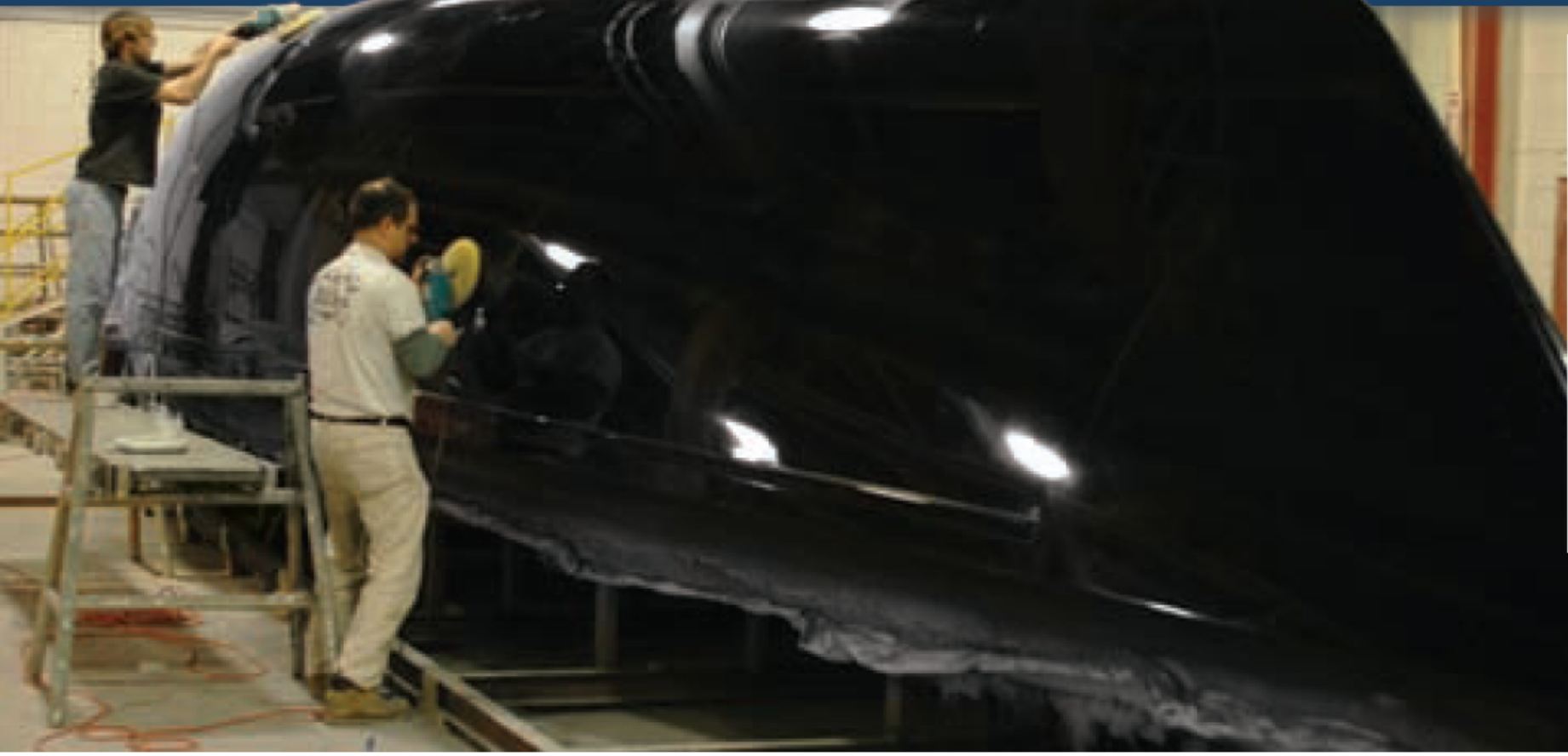
The plug is polished before being used to make the mold (above). A rugged weldment reinforces the mast partners (top right). Rudder bearing loads (right) are transferred via a star-shaped grid.
