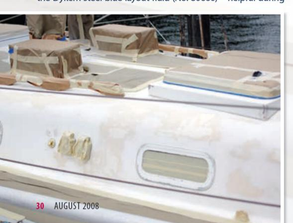
the filling process. The dye reveals areas that need to be filled or further sanded. Scratches and gouges should be filled with a sandable fairing compound like those from Interlux, System Three, and West System.
