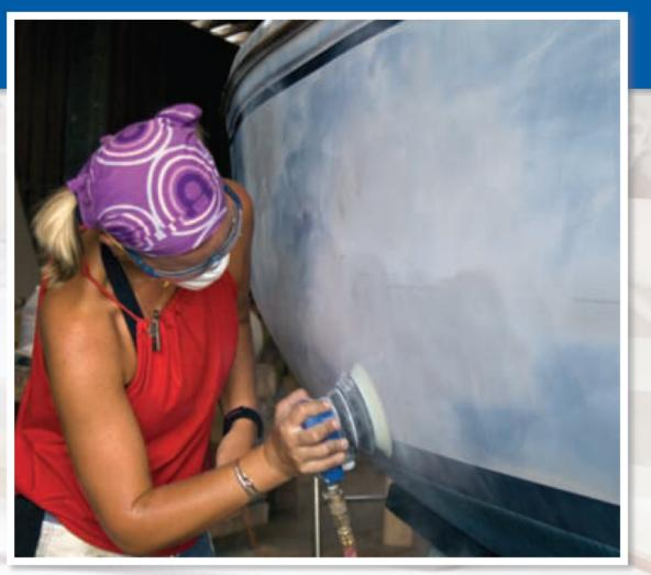
Applying blue dye to the hull highlights areas that need to be filled and further sanded for an even finish.
