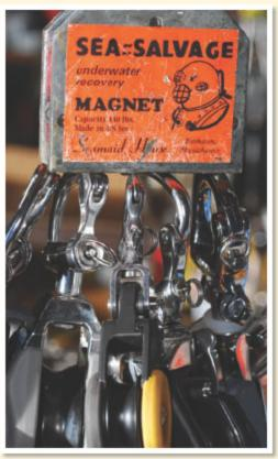
Although less resistant to corrosion than 316 stainless, the hardened magnetic, martensitic stainless steel in the snap shackles is stronger.
