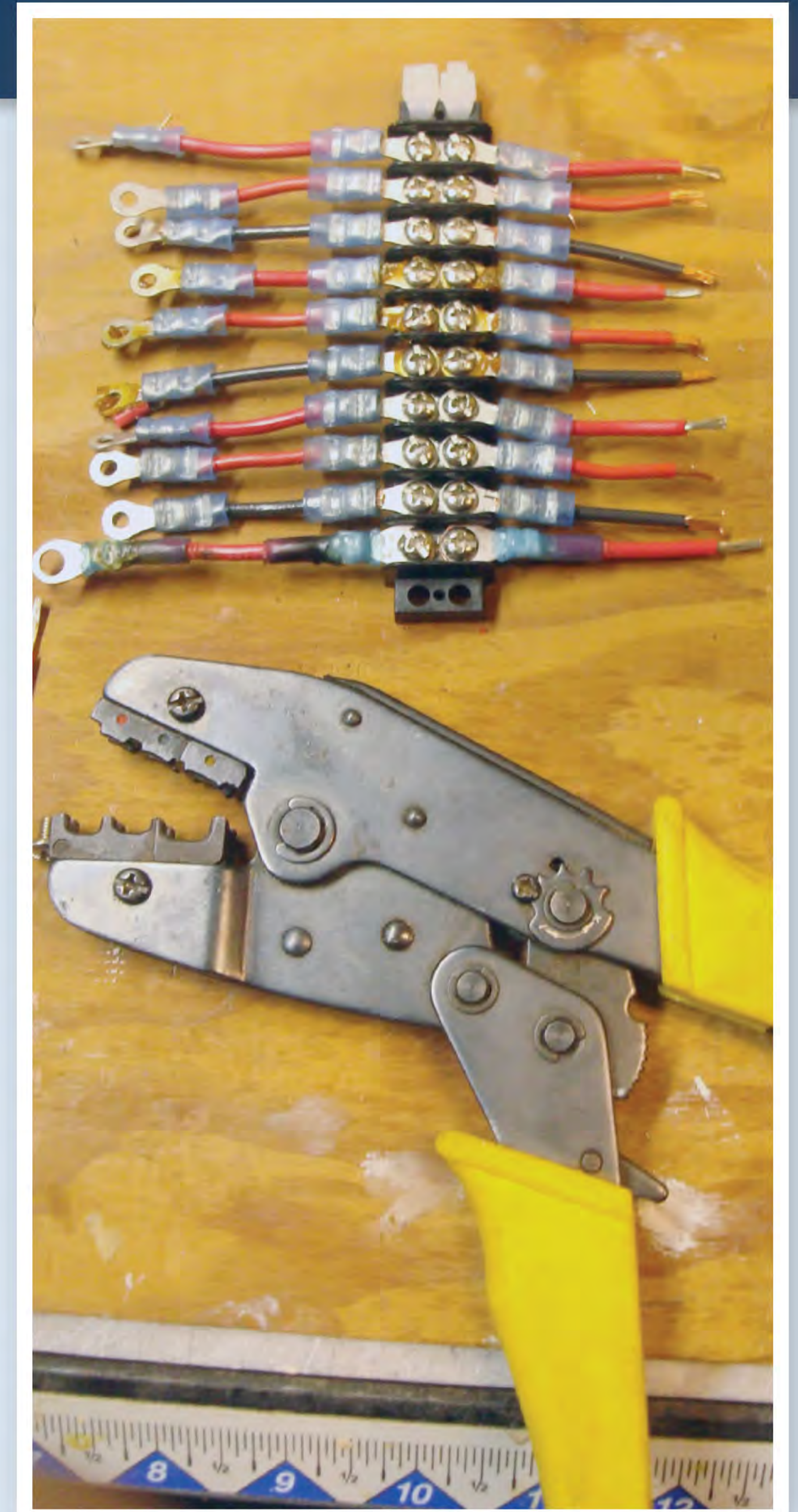
Used properly, a good-quality ratchet-style crimper offers consistent crimps that resist corrosion.
