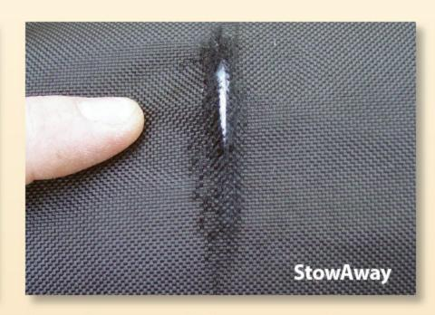
Testers used a rasp to evaluate the fenders' abrasion resistance. The Easystow showed minimal damage with just a few scratches on the cover, while the Aere' fender had little to no damage. The StowAway's nylon cover, however, wore all the way through to the bladder, proving it to be the least resistant to abrasion.
