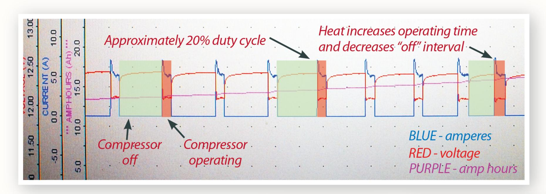
The graph above shows how the compressor reacts when heat is added. The compressor turns on more frequently and stays on longer, consuming more amphours. Frigoboat's manual controller (immediate right) and Smart Speed Control (far right) proved helpful to maximizing efficiency.
