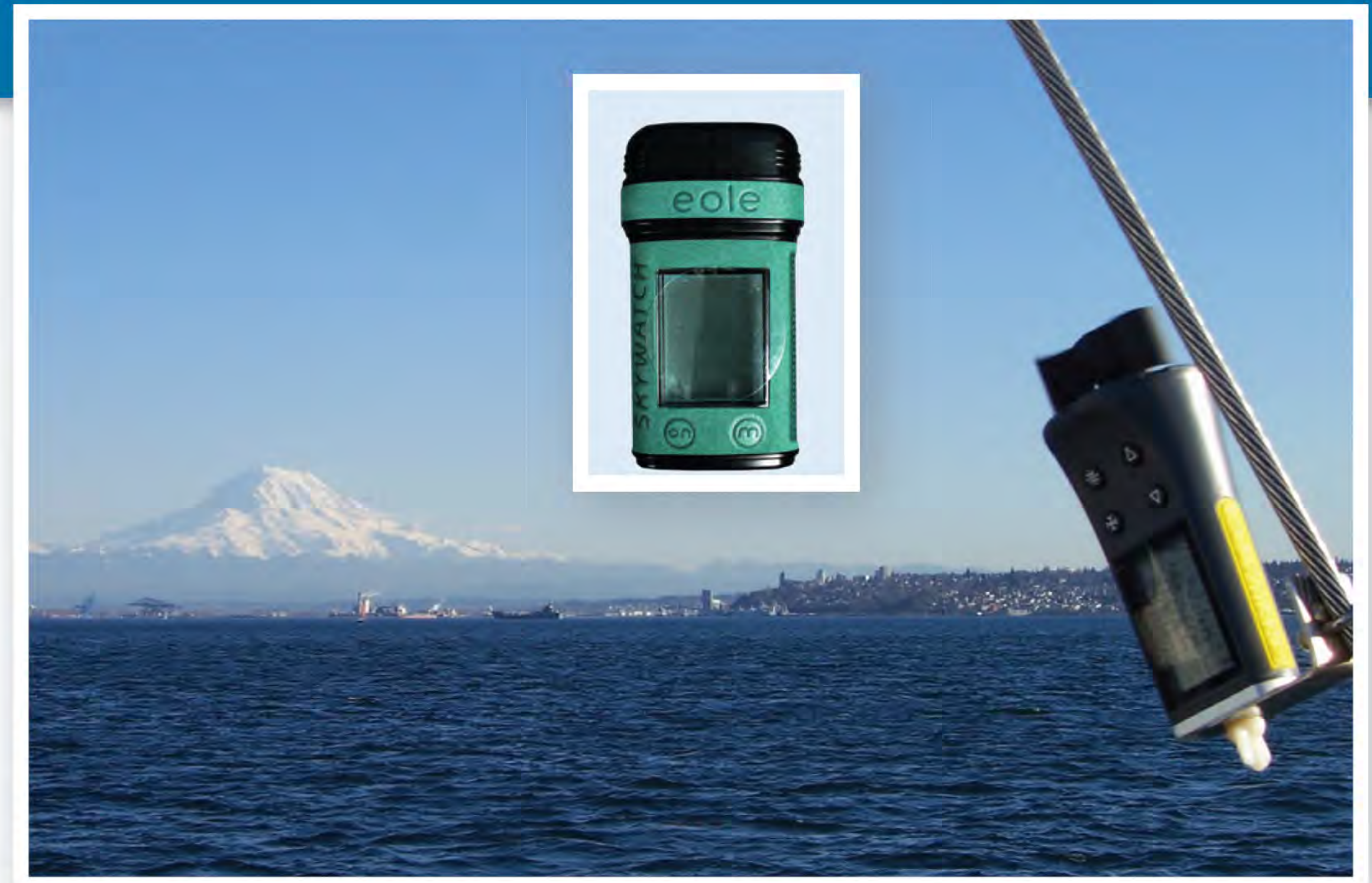
Mounted on a stay or shroud, the new Skywatch Eole and its predecessor (inset) can operate as handsfree wind meters. However, this setup isn't ideal for taking wind readings as they will be affected by the mainsail and a bimini or dodger.
