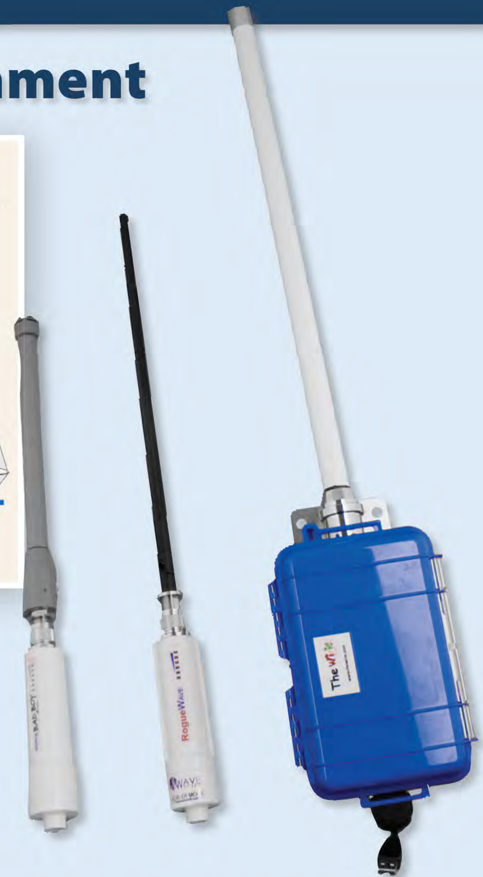
The Bad Boy Xtreme (6 dBi, left), the Rogue Wave (9 dBi, middle), and The Wirie (8.5 dBi, right) opt for broader omnidirectional radiating pattern to achieve reliable reception. The illustration above (adapted from one provided by Bitstorm) shows how a long-distance high-dBi antenna might not work as well when it is close under a marina transmitter.
