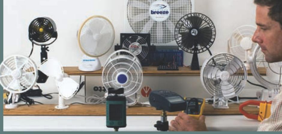
of a particular fan. While not getting into the science of propellers, it was obvious that some fans were more efficient in moving air at a given rpm, and that the number, size, twist, and shape of the blades had a lot to do with it. Current was measured with an Actron digital multimeter with accuracy +/- 1.2 percent.
