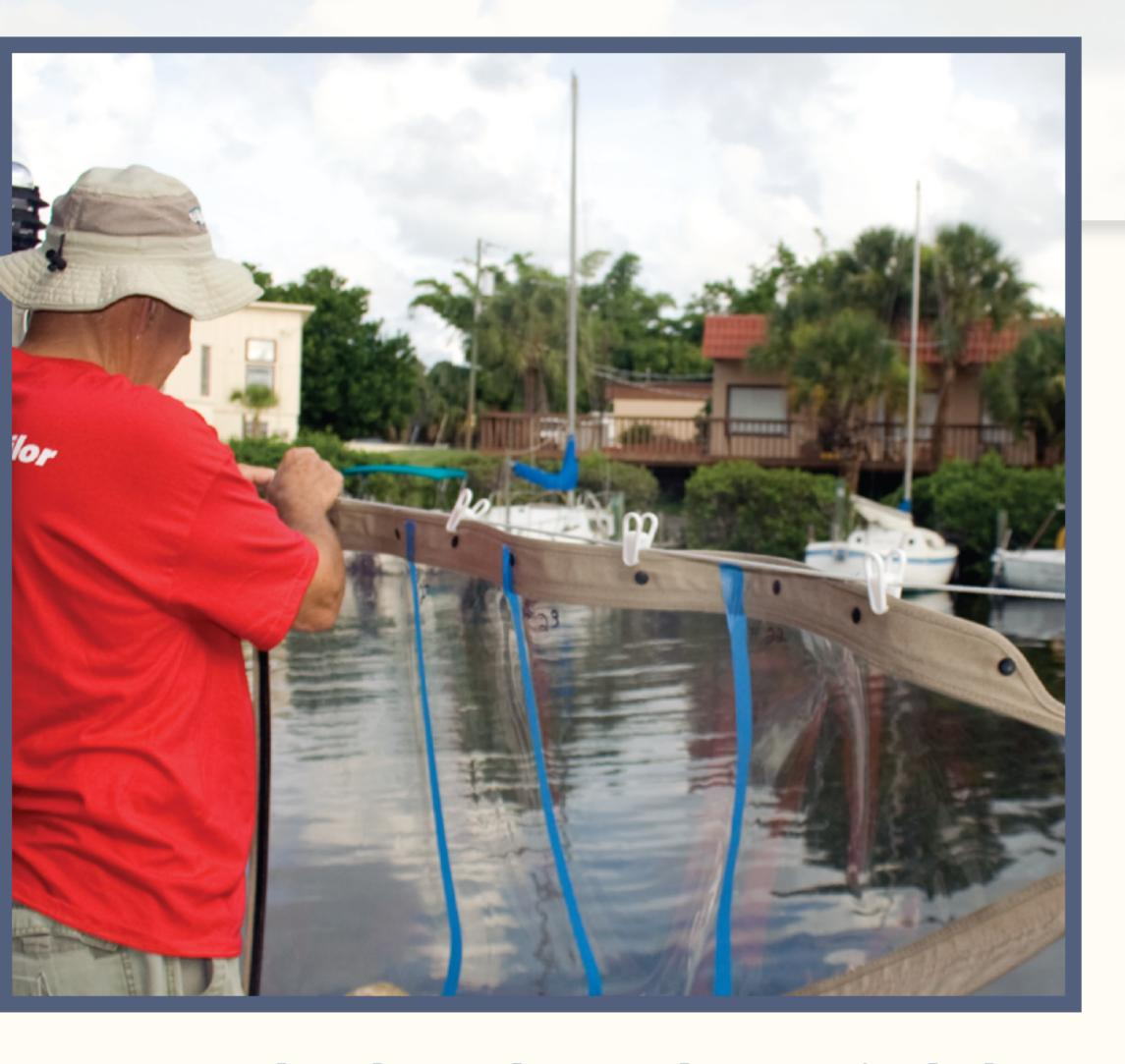
The clear-plastic cleaners/polishes test panel was left in the sun and salt air to weather for 30 days.
