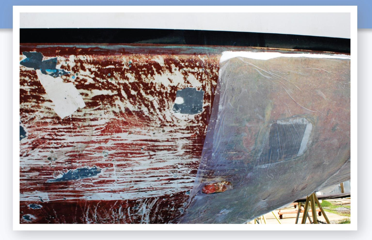
A 1-mil sheet of plastic was used to cover the Soy Strip to keep the chemicals from drying out. Peel Away recommends its own paper or regular butcher paper.
