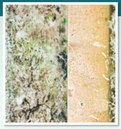
PS's past tests have found that ecofriendly paints wax and wane in effectiveness, just as most copperbased paints do. One 'green' paint, Microphase PhaseCoat UFR (above left panel), failed during our tests and has been pulled off the market.
