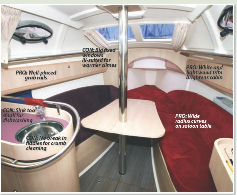
With a compact shower/head, a dedicated nav station, small galley, and an aft berth, the Etap 28s is set up well for family coastal cruising. The boat nevertheless takes an offshore approach to details like fiddles and grab rails. The use of lighter woods gives the boat a bright, uncluttered look.
