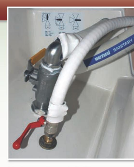
The inner and outer hull skins are brought together at all through-hull penetrations. However, the decision not to use long-lived silicon bronze seacocks is a step in the wrong direction, in our opinion.
