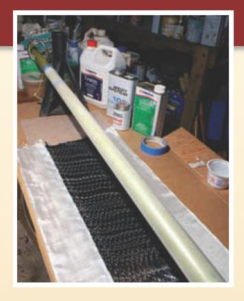
A tapered alloy windsurfer mast was used as a mandrel to build a carbon-fiber bowsprit for onthe-water furler testing. Forespar's aluminum sprit (right) is among several sprit options available off the shelf.
