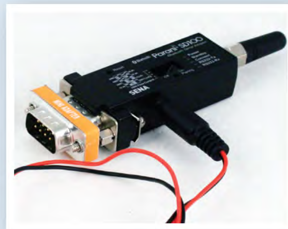
A Bluetooth dongle (above) links the PDA (right) to the boat's network. The Sail Clever software graphically displays performance data.
