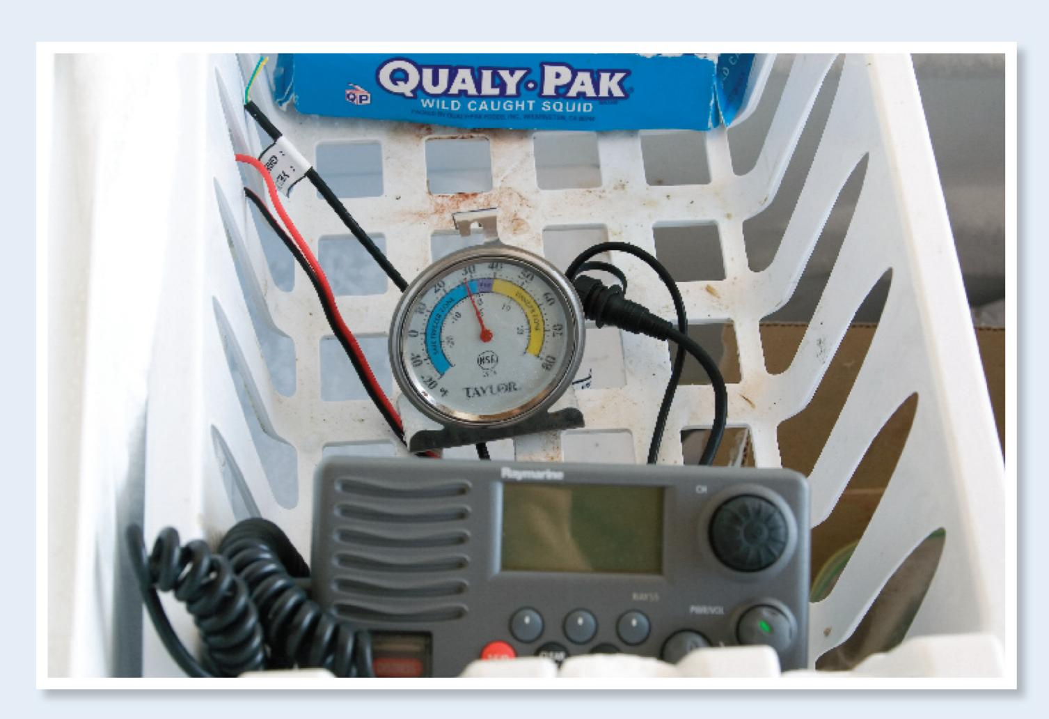
Testers used a bait freezer set at 15 degrees to simulate cold-weather extremes.
