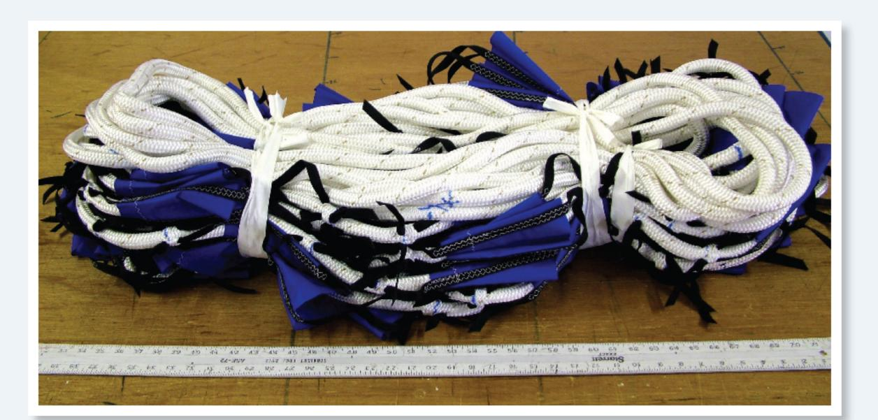
The crews of Hawk and Wind Horse (top photo) deploy a Series drogue for testing in calm waters. The Series consists of many small cones made from parachute material tied into a long warp (center). Tightly bundled, the Series can be easily stowed (bottom).
