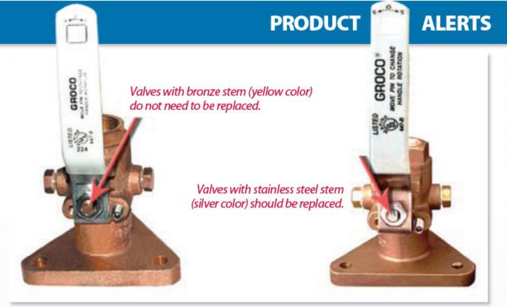
Groco is asking customers to check the valve stem on Groco seacocks. Those with a stainless stem (silver in color) should be replaced.
